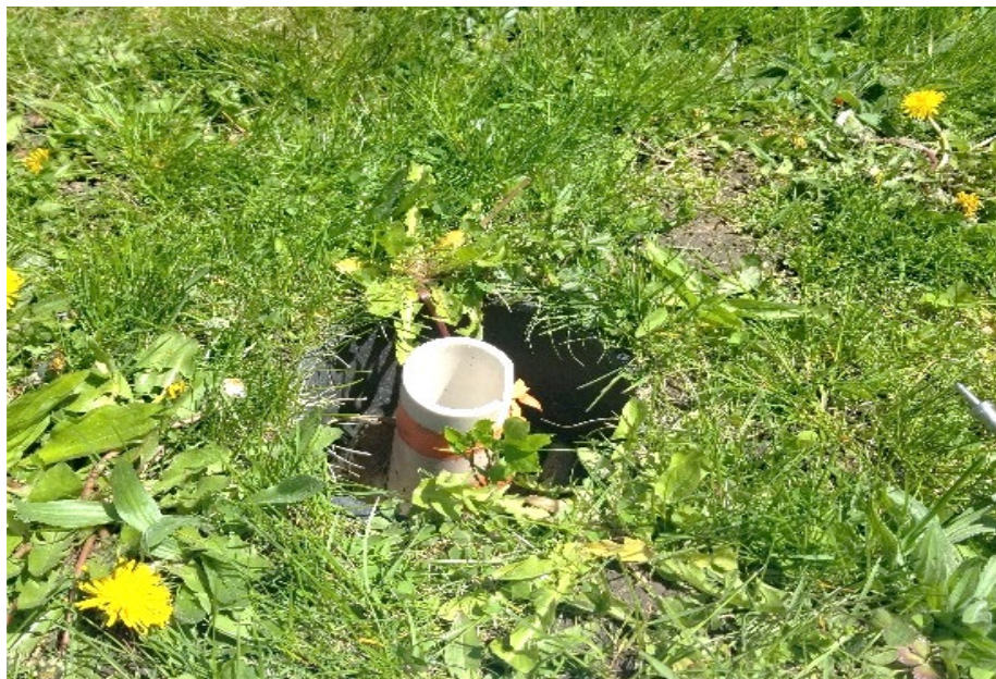
Photograph of soil gas monitoring point SP-7R on April 29, 2022. A metal sampling point was located inside the PVC pipe, though both the PVC and sampling point were loose. Roughly a 6-inch diameter hole had been advanced, which was partially filled with coarse sand and pea gravel, but no seal was observed.
